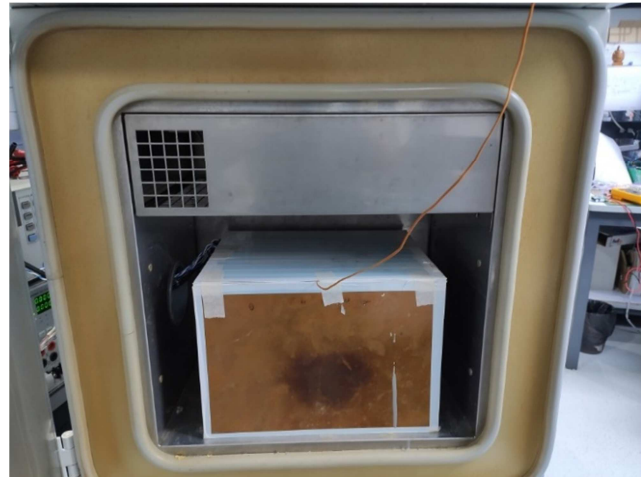
Figure 105 – Thermal Performance Set-up Using Thermal Chamber.
