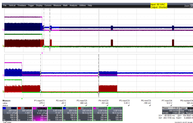
Figure 105 – Output Voltage and Current Waveforms. 90 VAC Input. Output Shorted. Upper: LNK-XT2SR_V DS . 200 V / div. Upper Middle: 5 V OUT , 1 V / div. Lower Middle: 12 V OUT , 5 V / div. Lower: LNK-XT2SR_I DS , 500 mA / div. 500 ms / div. Zoom: 50 ms / div.
