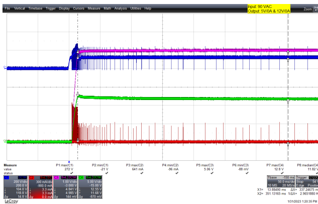
Figure 85 – Drain Voltage and Current Waveforms. 90 VAC Input, No-Load. Upper: LNK-XT2SR_VDS. 200 V / div. Upper Middle: 5 V OUT , 1 V / div. Lower Middle: 12 V OUT , 5 V / div. Lower: LNK-XT2SR_IDS, 300 mA / div. 5 ms / div.
