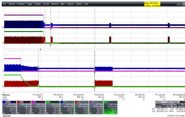
Figure 103 – Output Voltage and Current Waveforms. 90 VAC Input. Output Shorted. Upper: LNK-XT2SR_V DS . 200 V / div. Upper Middle: 5 V OUT , 1 V / div. Lower Middle: 12 V OUT , 5 V / div. Lower: LNK-XT2SR_I DS , 500 mA / div. 500 ms / div. Zoom: 50 ms / div.
