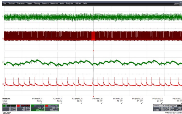
Figure 113 – Output Ripple Voltage Waveforms. 90 VAC Input. 5 V PK-PK : 32 mV, 12 V PK-PK : 91 mV. Upper: 5 V OUT , 20 mV / div, 5 ms / div. Lower: 12 V OUT , 50 mV / div, 5 ms / div. Zoom: 100 μs / div.
