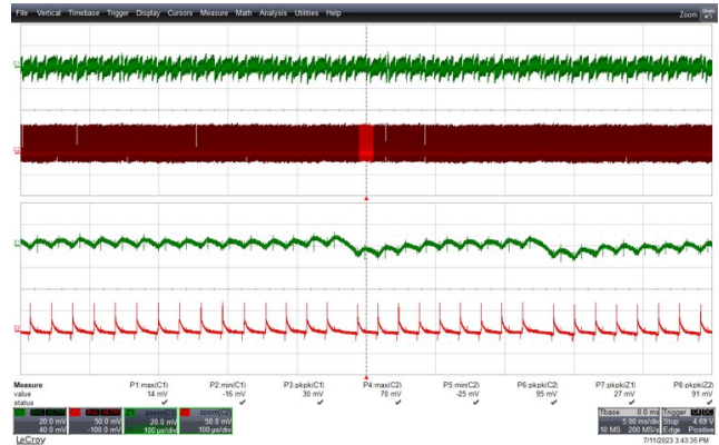
Figure 114 – Output Ripple Voltage Waveforms. 265 VAC Input. 5 V PK-PK : 30 mV, 12 V PK-PK : 95 mV. Upper: 5 V OUT , 20 mV / div, 5 ms / div. Lower: 12 V OUT , 50 mV / div, 5 ms / div. Zoom: 100 μs / div.
