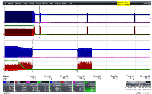
Figure 104 – Output Voltage and Current Waveforms. 265 VAC Input. Output Shorted. Upper: LNK-XT2SR_V DS . 200 V / div. Upper Middle: 5 V OUT , 1 V / div. Lower Middle: 12 V OUT , 5 V / div. Lower: LNK-XT2SR_I DS , 500 mA / div. 500 ms / div. Zoom: 50 ms / div.
