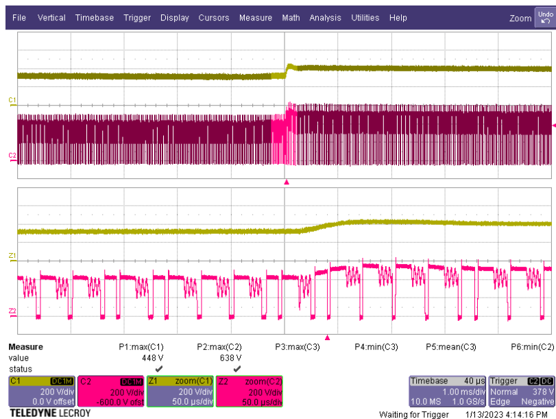
Figure 148 – 230 VAC, +1 kV, Differential Surge L-N
