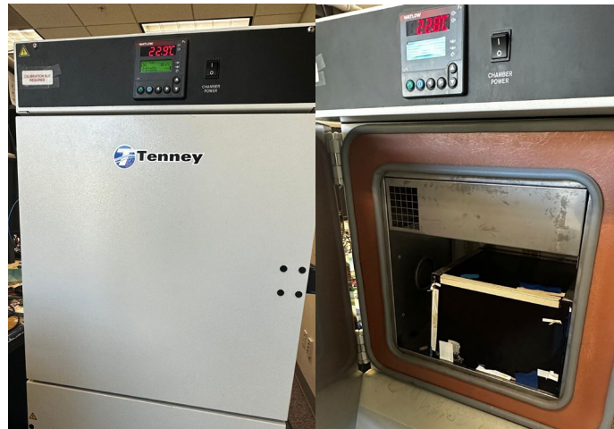
Figure 56 – Thermal Chamber Test Set-up.
